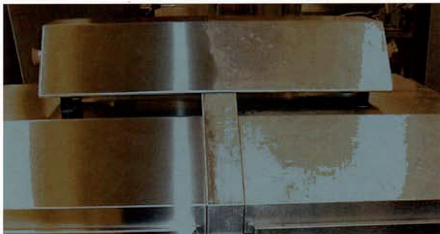
This image shows a unit where the left hand side was coated with \text{NPSiO}_2 but the right hand side was not coated prior to use. After use both sides were cleaned with water
